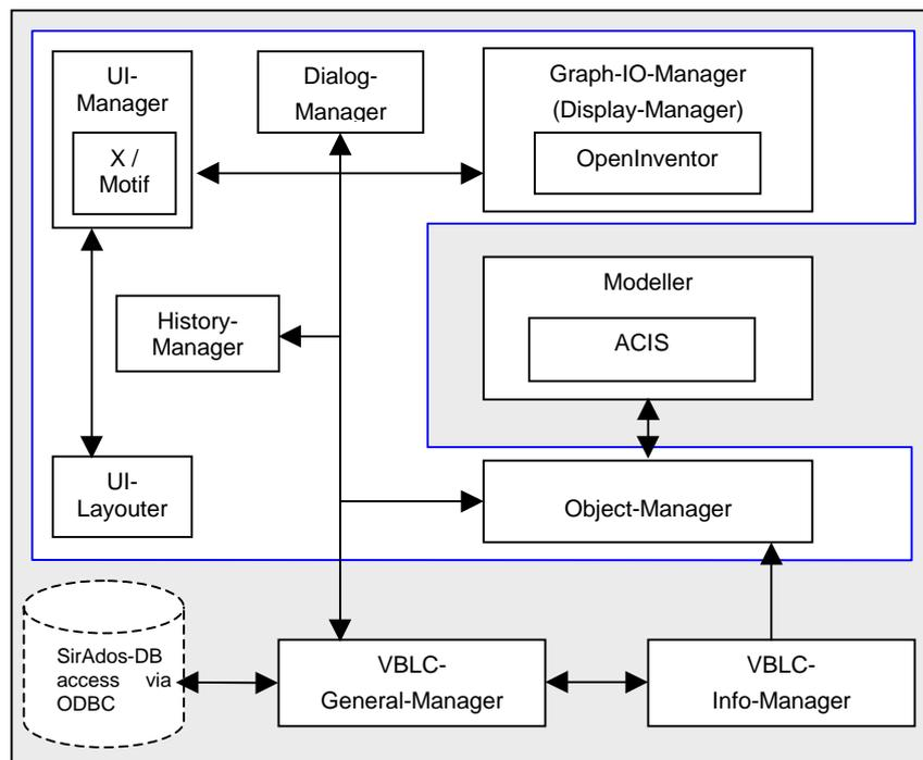
Figure 1: System architecture of ARCADE with VBLC.
